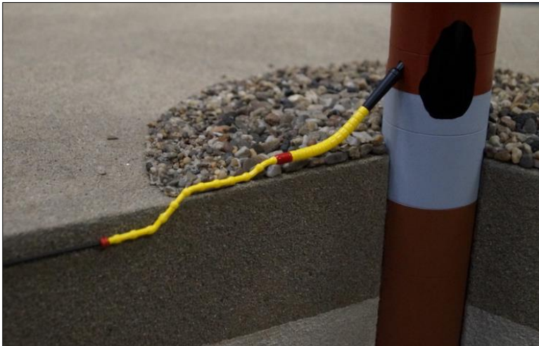
Figure 7-5 Monopile and anti-scour protection (OWF Gemini)
